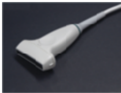
75L60EA Linear Application: Orthopedics, Breast, Musculoskeletal
