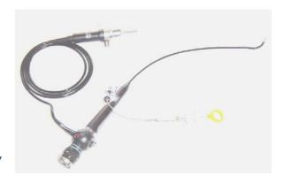
There are fluid filling, ware ring and suction valves built in at the operating handle. With the advantage of large aperture diameter of forceps channel where even if instrument is handling, fluid filling, watering and suction may be proceeded as well.
