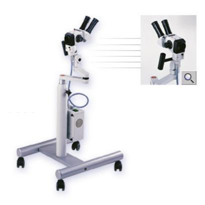
An optional video camera can be integrated enabling co-observation as well as documentation via video tape recording or computerization.
