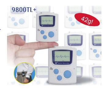
After recording, the data recorded in the recorder will be uploaded to PC through USB cable
